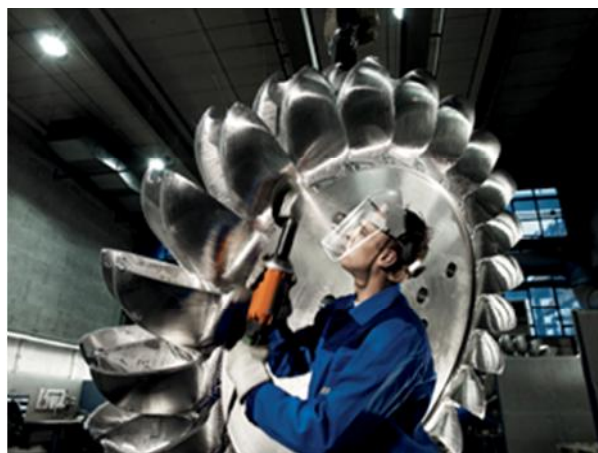
Manufacturing hydro power turbines (Photo: Andreas Hofer /ANDRITZ HYDRO)
